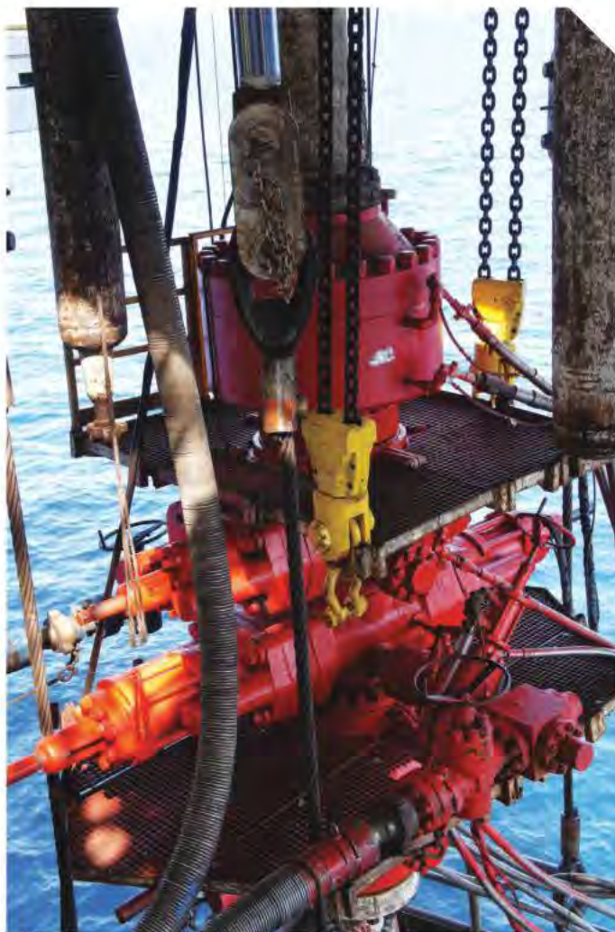
At the heart of the matter: a blowout preventer. Photo from iStock.
