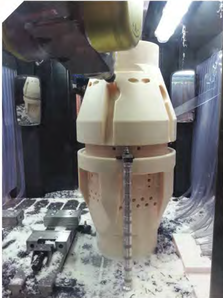
Nylacast component being machined. Images from Nylacast.
