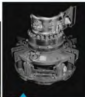
A wellhead connector, shown from data a subsea laser scan.
