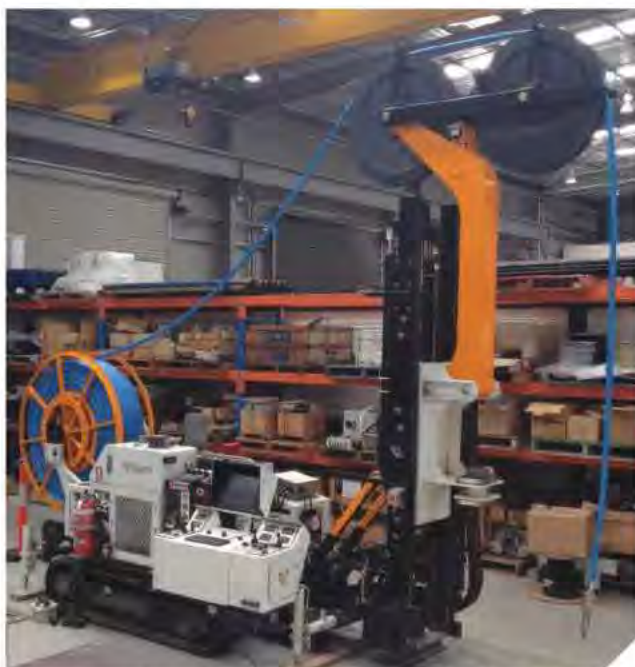
The coiled tubing drill rig prototype modified for use with flexible H-Coil, a potentially more durable, alternative to steel tubing, last year. Photo from Deep Exploration Technologies CRC.
