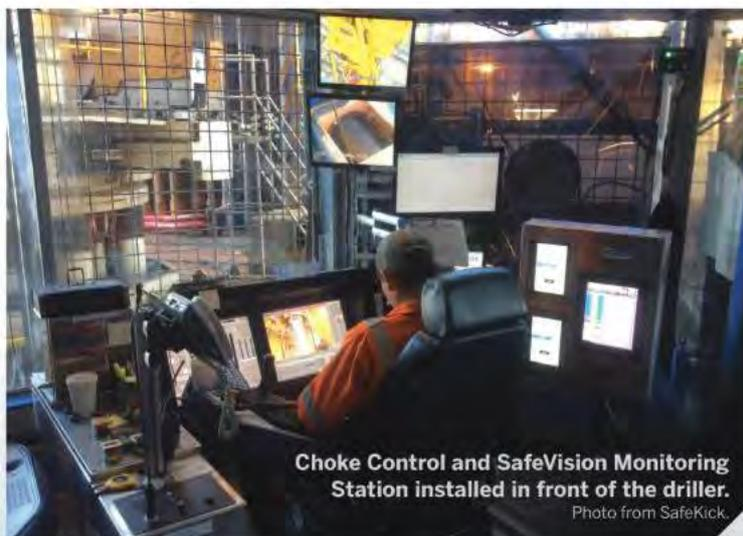
Choke Control and SafeVision Monitoring Station installed in front of the driller.
