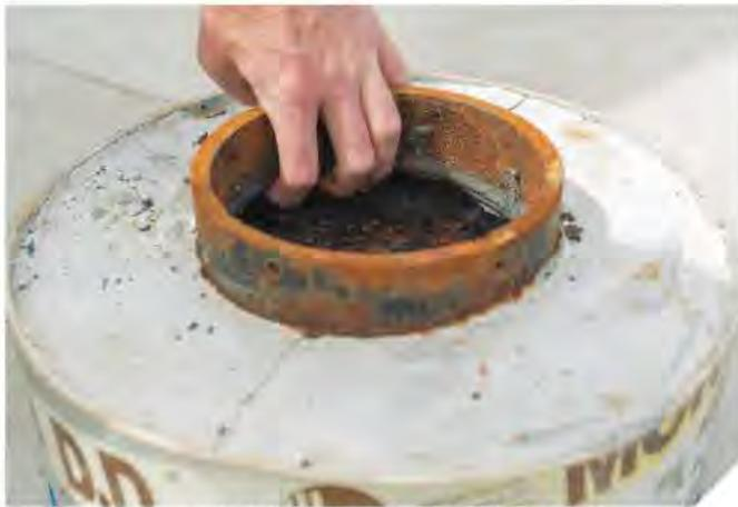
Casing and cement string after plasma milling testing.
