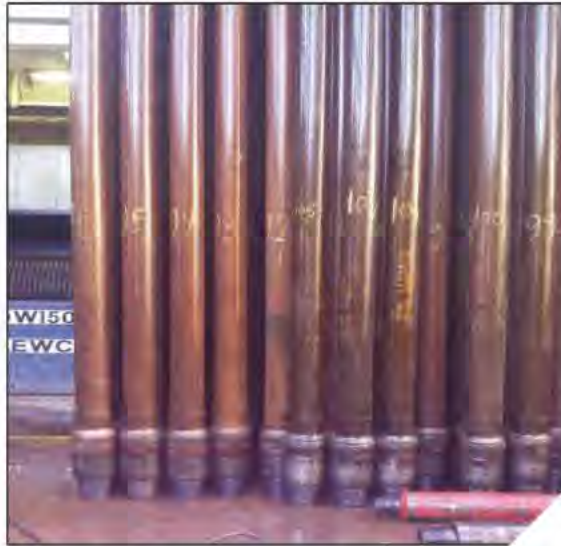
An example of a successful displacement is recognized by bright, clean pipes indicating clean casing and fluid. Photo from Halliburton.
