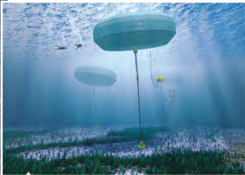
A Ceto array. Image from Carnegie Wave Energy.
