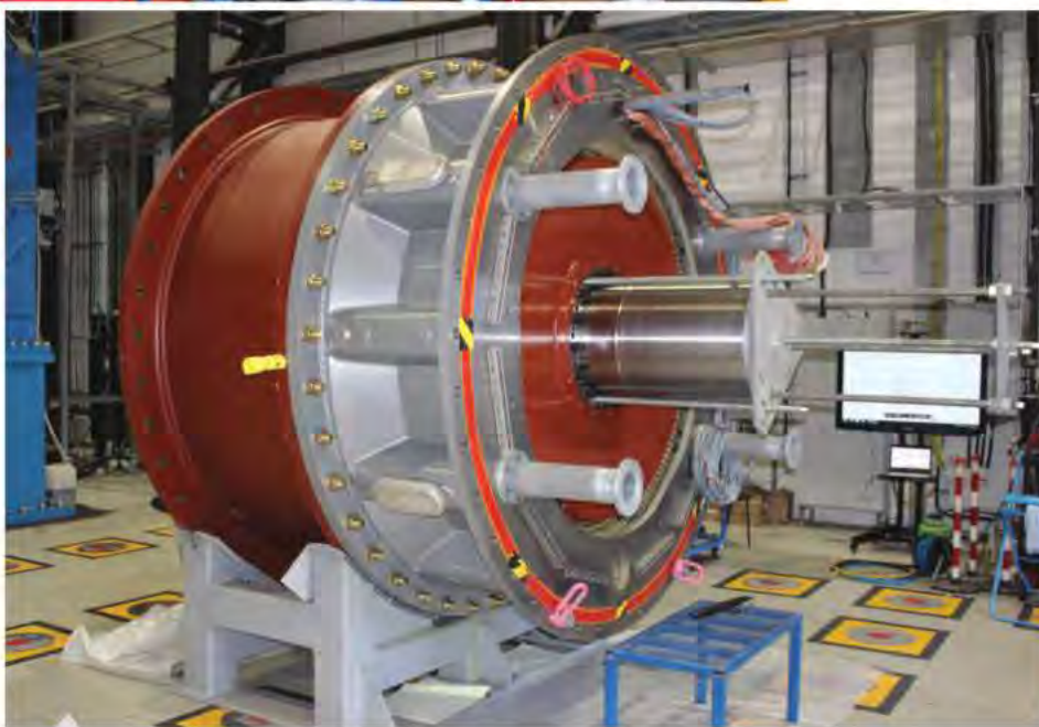
An AR1500 generator and gearbox being assembled at OREC. Photo from Atlantis Resources.
