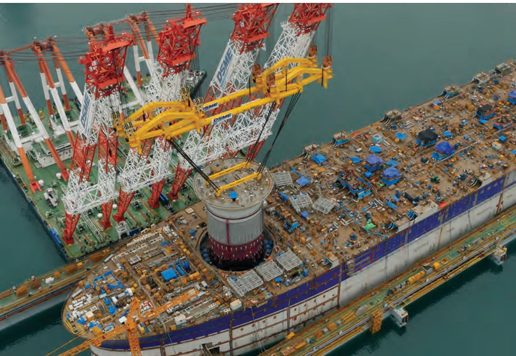
The Ichthys turret being lowered into the FPSO in November 2014. Photo from SBM Offshore.
