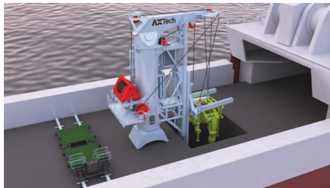
AXTech's light module handling system, Middle position in moonpool. Images from AXTech.
