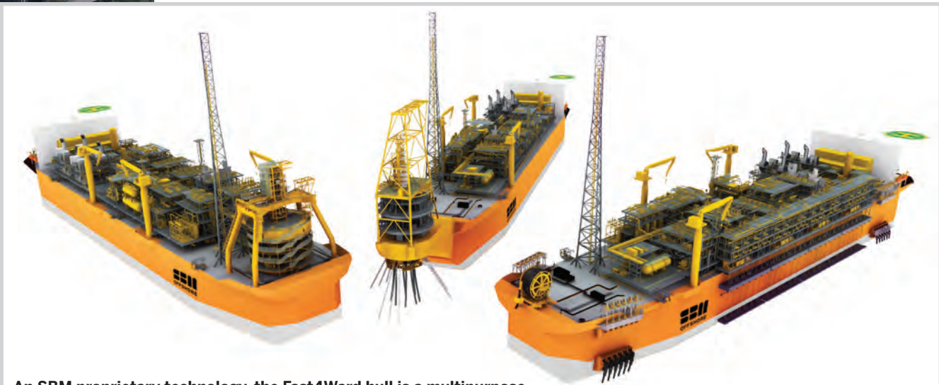
An SBM proprietary technology, the Fast4Ward hull is a multipurpose floater and has the versatility to receive various large topsides with spread or turret mooring configurations. It comes fully outfitted with all the necessary marine, utility and cargo systems and with an accommodation block and bridge.
