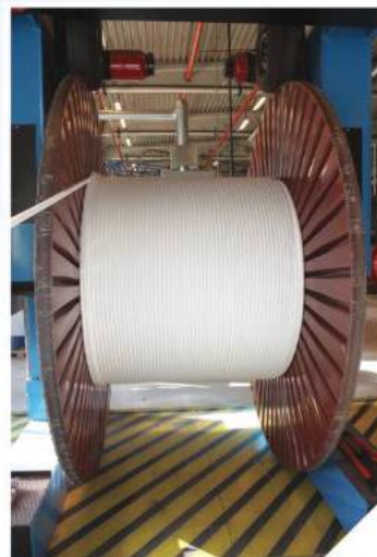
Carbon fiber, from bobbin to umbilical. Photos from Nexans.
