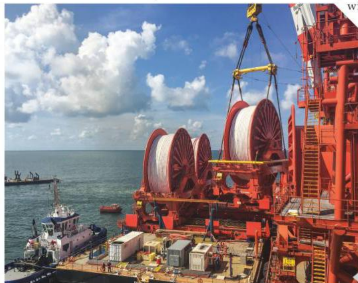
Reel exchange offshore.
