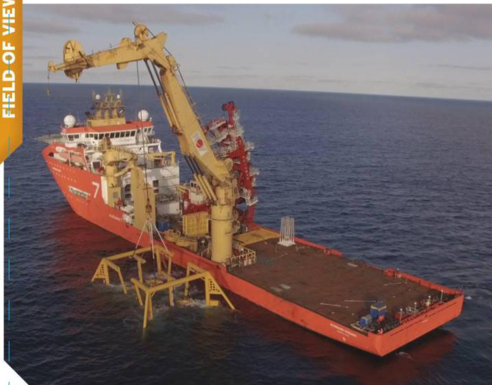
A Maria template close to installation with the Normand Oceanic .
