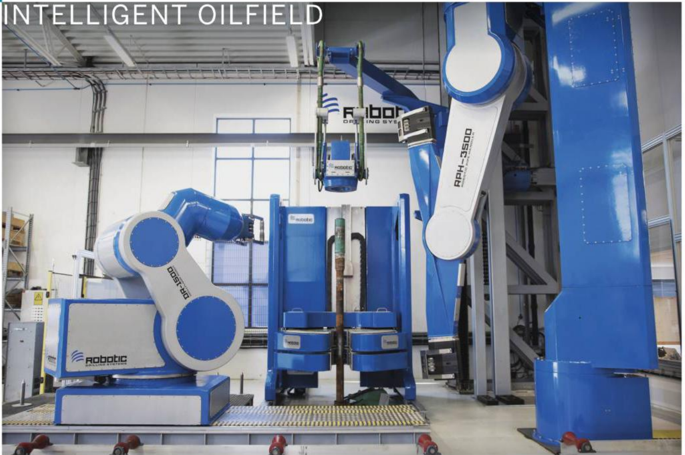
The full robotic drill floor system during workshop testing. Photo from RDS.
