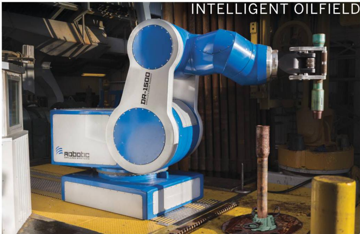
The world's first drill floor robot installed at the Ullrigg Drilling and Well Centre. Photo from RDS.
