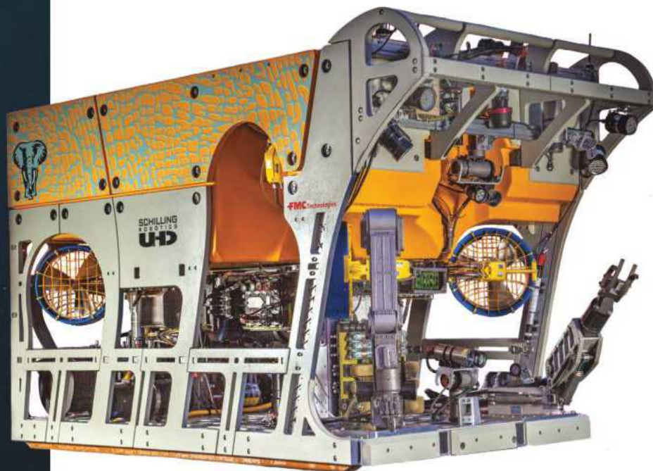
The UHD Gen III ROV. Photo from FMC Technologies.
