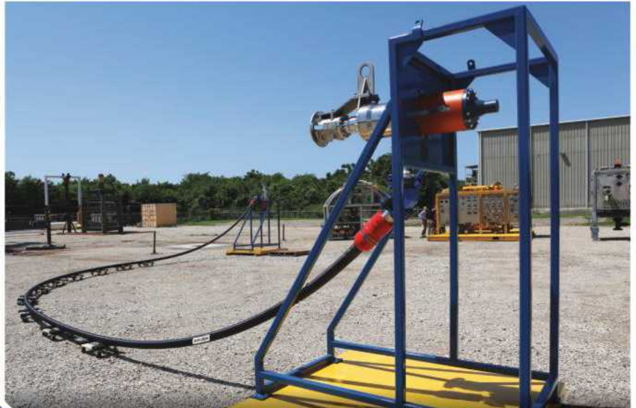
Magma's 2in jumper being put to the test at Oceaneering's facility in Houston.
