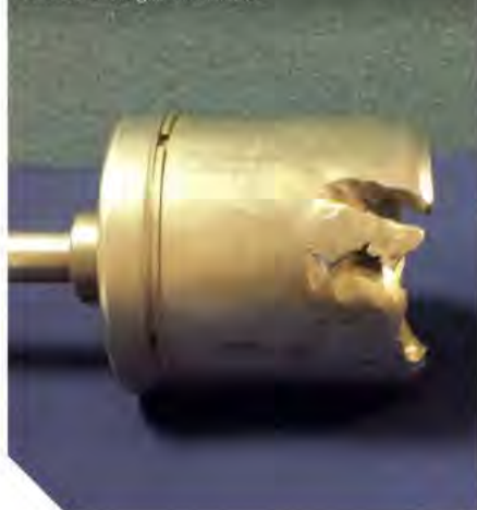
Counting the cost: sand eroded choke valves. Images from NEL.
