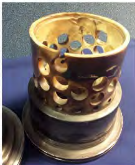
Counting the cost: sand eroded choke valves. Images from NEL.
