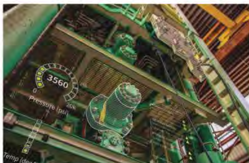
The BOP has an overlay showing the status of the component. Photo by Katy Weintritt; provided by NOV.
