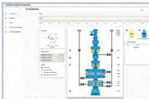
NOV's customer portal for BOP condition monitoring. Images from NOV.
