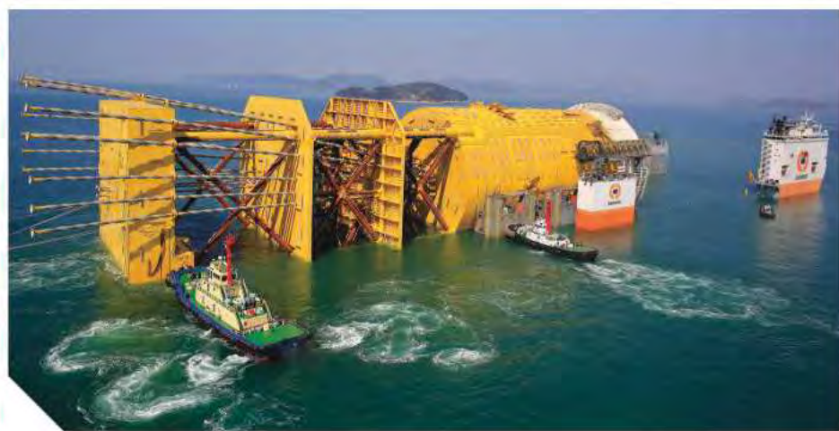
Above and left: Statoil's Aasta Hansteen spar being loaded onto the Dockwise Vanguard in South Korea, late April. Images from Statoil.
