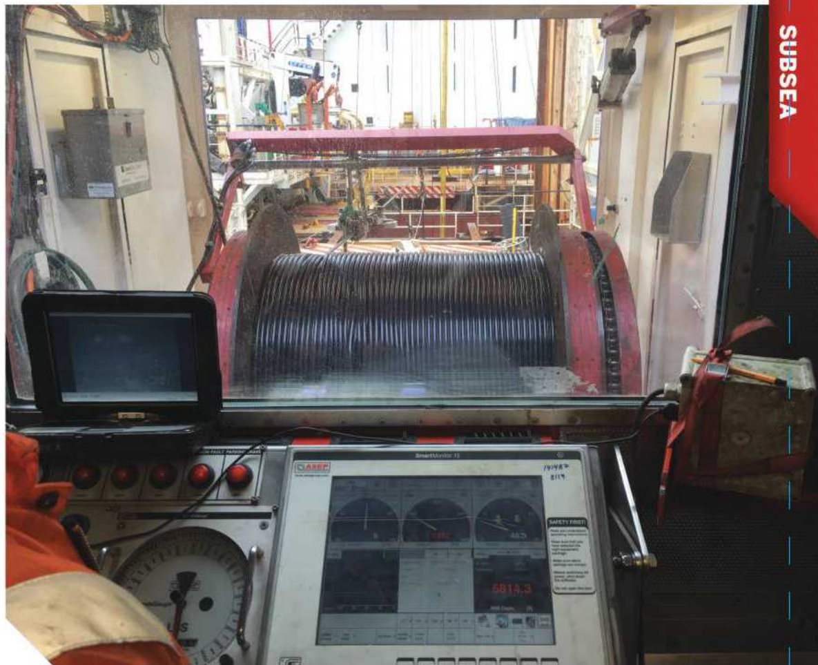
Coilhose being deployed on board the LWIV.
