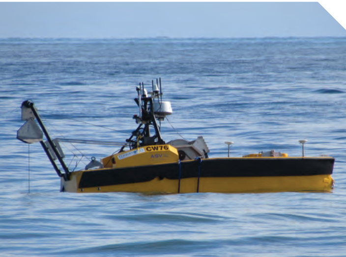
ASV Global's C-Worker 5 on a cable route survey, with TerraSond. Photo from ASV and TerraSond.
