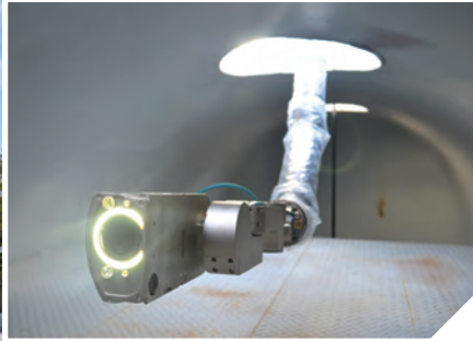
Last year, Chevron tested a snake-arm robotic inspection system, the P100 from OC Robotics, to inspect inside pressure vessels on its assets in the North Sea, following onshore trials. Image from OC Robotics.
