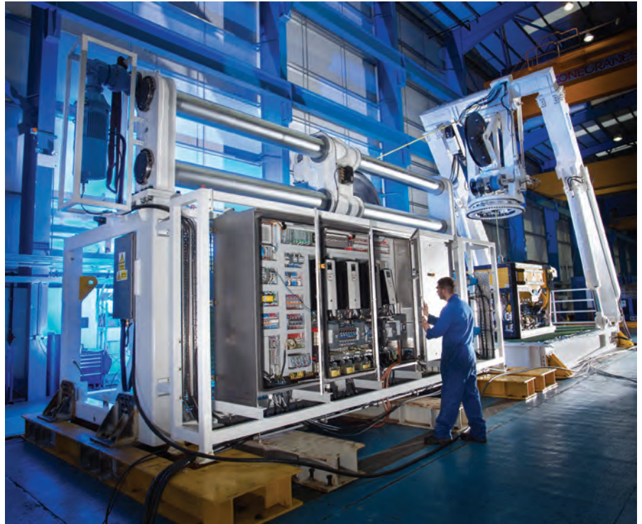
A 6000m Quasar Work Class ROV system, from SMD, which was supplied to Shanghai Salvage, with SMD’s firm’s first electric winch, late 2017.
