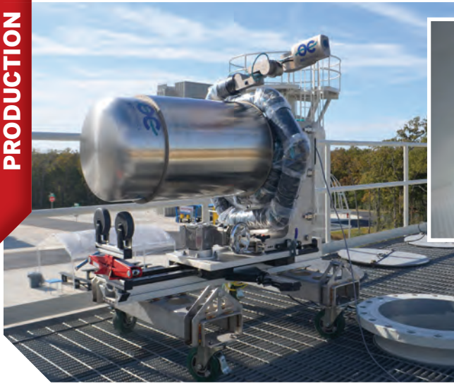
Last year, Chevron tested a snake-arm robotic inspection system, the P100 from OC Robotics, to inspect inside pressure vessels on its assets in the North Sea, following onshore trials. Image from OC Robotics.
