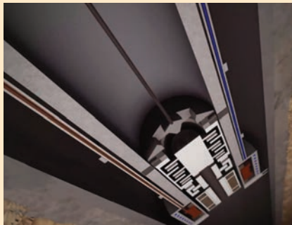
Upwing Energy's MDS, with hermetically sealed electrical components outside of the tubing.
