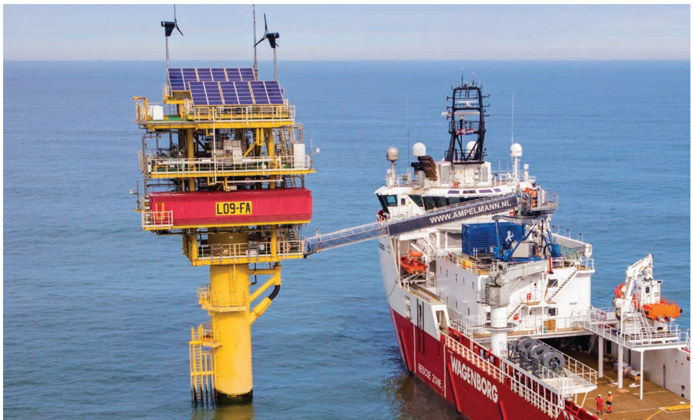
Ampelmann's gangway systems can be used for transfers to both fixed and floating installations.
