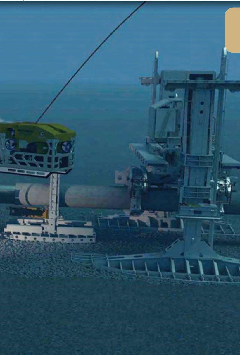
The world's only fully remote diverless pipeline (MIG) welding equipment spread, including the habitat, H-Frames, and remote welding tool.
