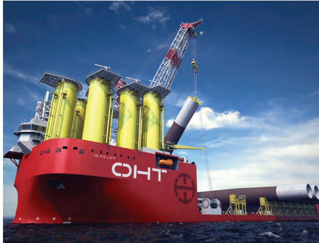
*The 216-meter long Alfa Lift vessel will feature a 3000-tonne crane and will be capable of carrying and installing up to 14 XL monopiles per voyage.*
